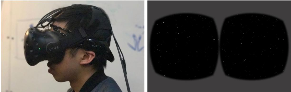
**Figure 1.** Left: A participant wearing HTC VIVE HMD and the EMOTIV Insight EEG BCI. Right: Visual stimuli of the virtual environment designed to provide optic flow but eliminate all visual landmarks.
