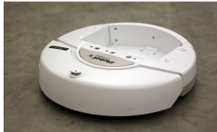
Figure 5.1: Out of the box iRobot Create
