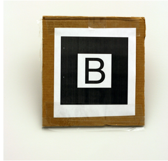
Figure 5.8: A wall-mounted ARtoolkit fiducial used for localization
