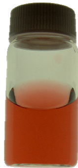
Figure 2.4 Aqueous solution of solid spherical gold NPs with white light illumination from behind the sample.
