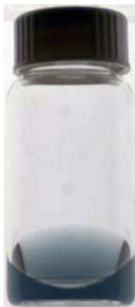
Figure 2.8 Aqueous solution of silica/gold core-shell NPs with white light illumination from behind the sample.
