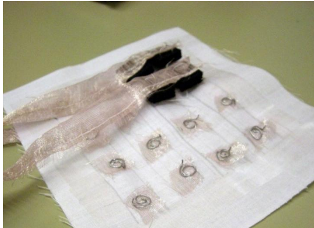
Figure A.10: A fabric touch pad made from conductive foam (black), diodes, and silk organza.
