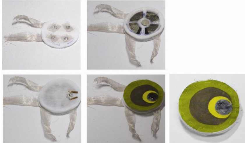
Figure 4.8: 4 layers of Patch electronics simplified from original design.
