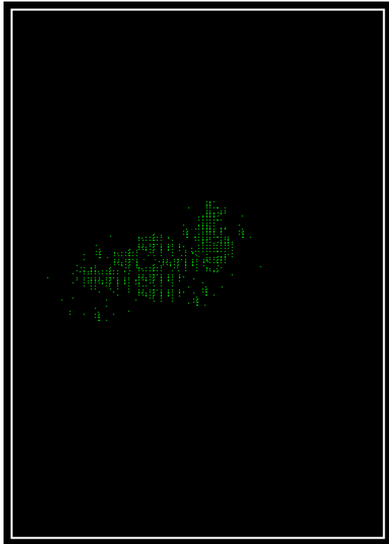
Figure 4.12: Network interface of 32-node star topology on Xilinx Virtex 5 LX330
