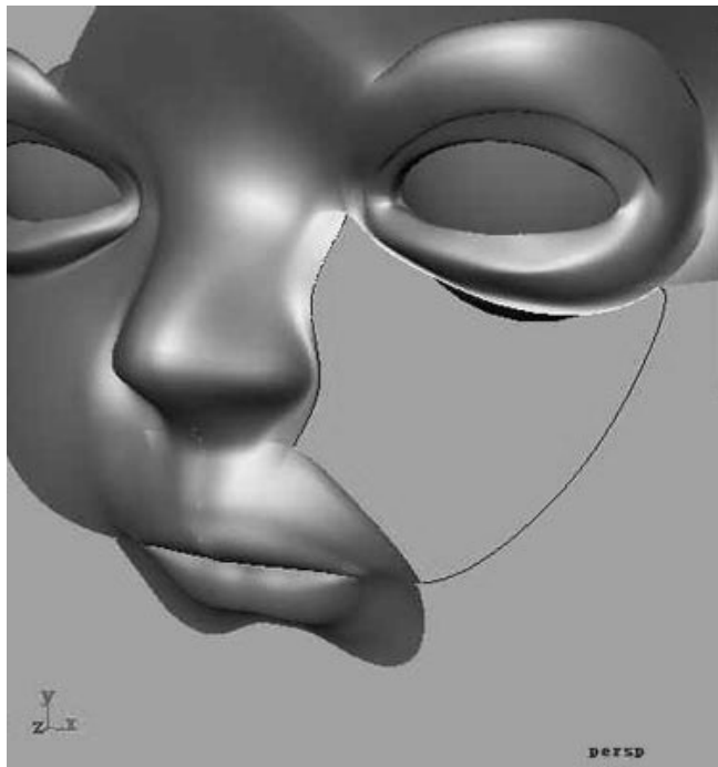
Figure 2-8 A baby's face modeled with NURBS patches. The blue curves compose one patch that covers the cheek of the face.
