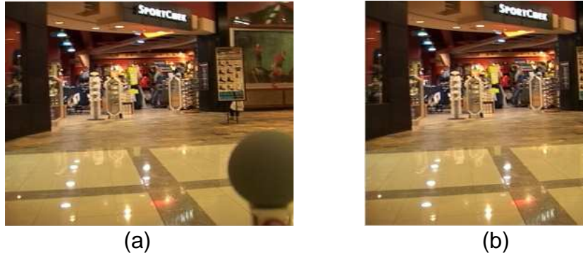
Figure 9.1 Example image from the dataset. (a) Original image containing gray ball from which the colour of the scene illumination is determined. (b) Cropped image to be used for algorithm testing with gray ball removed.
