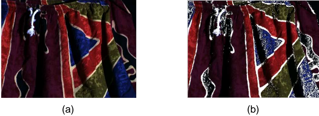
Figure 3.2 Gray-pixel Detection Results. (a) Input image; (b) Pixels identified as gray are indicated in white.
