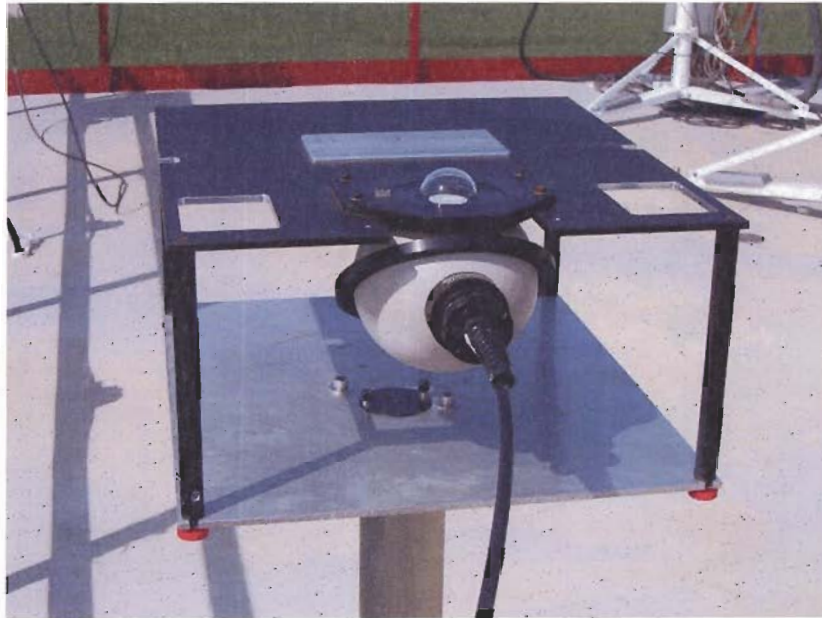
Figure 1.4. Photograph showing the integrating sphere of the Optronic Laboratories OL 754 Portable High Accuracy UV-Visible Spectroradiometer on a tripod. The spectroradiometer measures spectral global irradiance on the elevated platform at the Bratt's Lake Observatory.
