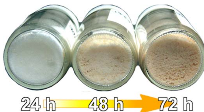
Figure 3.1 Color of the LiOPr i after 24, 48, and 72 h of synthesis by the metal redox method [equation (14)].
