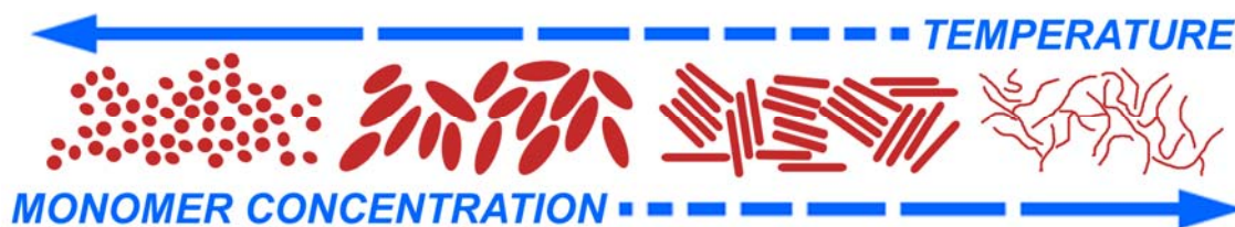
Figure 2.4 The kinetic and thermodynamic growth model contributing to (from left to right) nanocrystals, nanoeggs, nanorods, and nanowires. Technically, both the top and bottom axes can be considered “temperature.” They have been labelled this way to distinguish between excessive temperatures leading to a loss of surface energy anisotropy (top), and to the regular thermal increase in monomer production (bottom).
