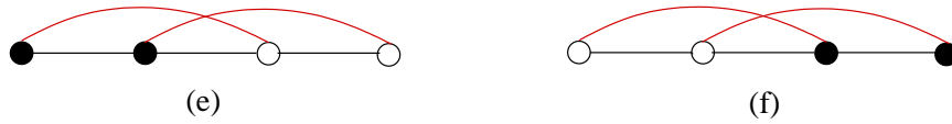
Figure 5.2: Allowed subgraphs in the optimal solution for the MDCVRP on a path.
