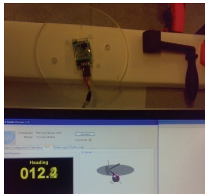
Figure 5.18: Heading angle with hard-iron disturbances (iron handle)
