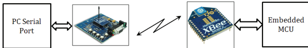
Figure 5.8: Wireless communication to the host PC using Zigbee™
