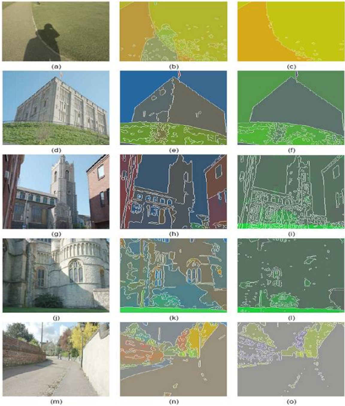
Figure 3.5: Input colour images (a,d,g,j,m), their chromaticity (b,e,h,k,n), and the chromaticity images for an extracted illumination invariant (c,f,i,l,o). Here, the Mean-Shift algorithm has been applied to generate a cleaner image, and edge-detection overlaid — the illumination invariant has fewer edges on shadow boundaries. Cameras used were an HP 912 and a Nikon D70.
