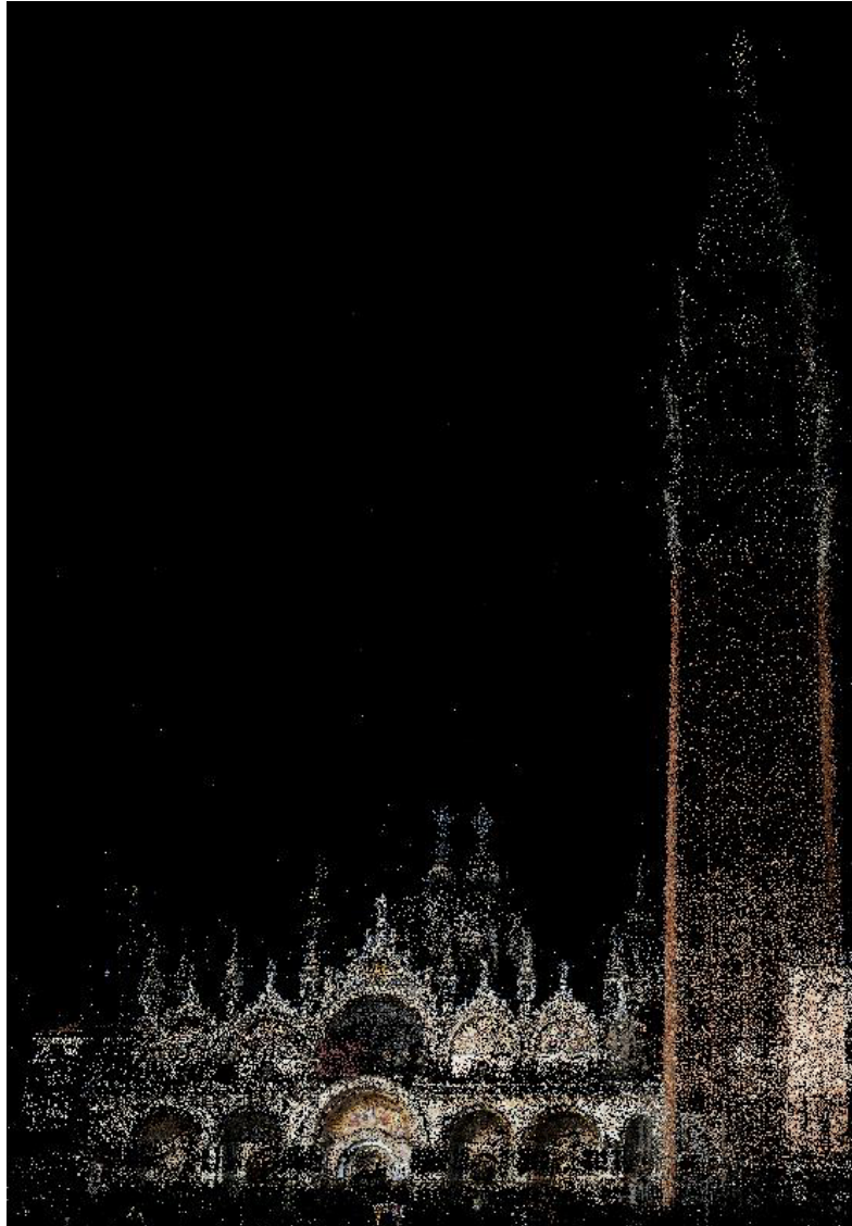
Figure 3: This is a point cloud of the Basilica di San Marco and Campanile di San Marco, as seen from the Piazza San Marco in Venice. It is composed of many individual dots. 9
