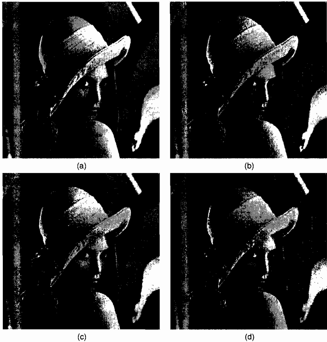
Figure 5.4: Reconstructed image Lena at R = 1/M bpp, 25% redundancy and different configurations. (a) D_{3,3} (39.25 dB). (b) D_{3,2} (34.57 dB). (c) D_{3,1} (31.36 dB). (d) D_{4,1} (29.45 dB).
