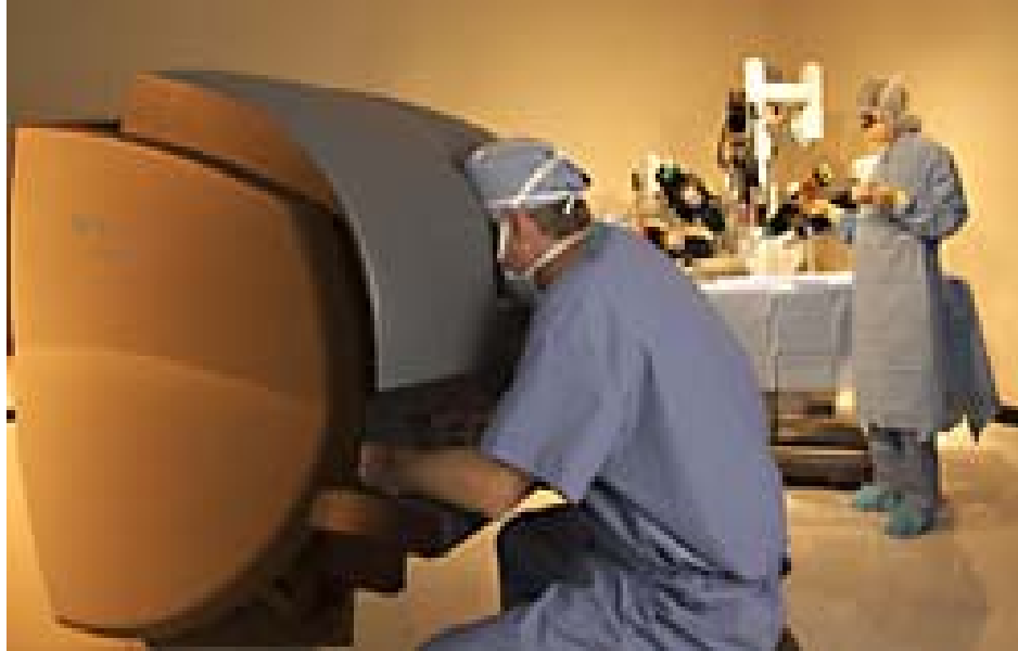
Figure 1.3: The da Vinci robot system for MIS
