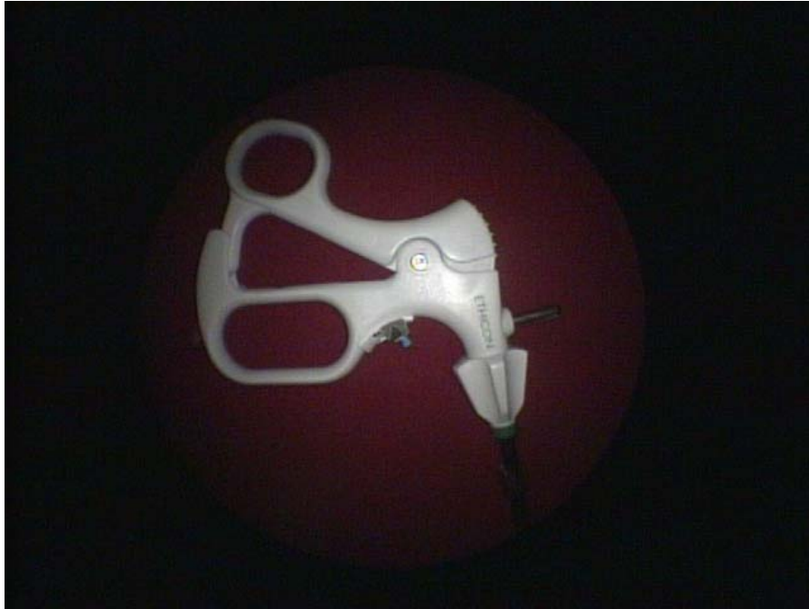
Figure 3.6: The wireless switch is attached to the handle of the surgical tool
