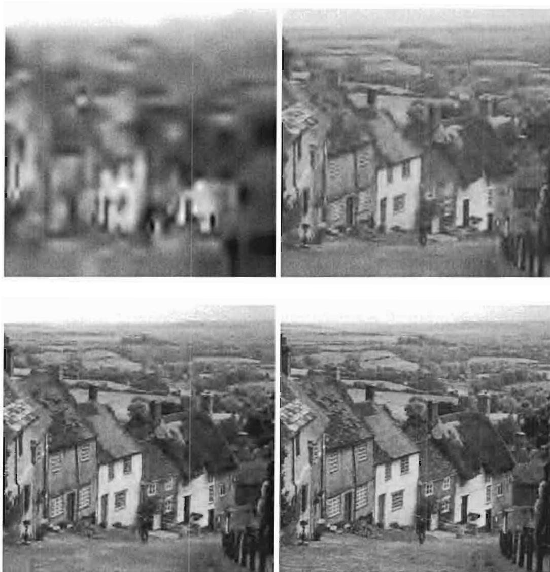
Figure 2-2. Four-layer quality-scalable Goldhill image decoded at the first layer with 0.01 bpp (top left), the second layer with 0.05 bpp (top right), the third layer with 0.1 bpp (bottom left), and the fourth layer with 0.2 bpp (bottom right).
