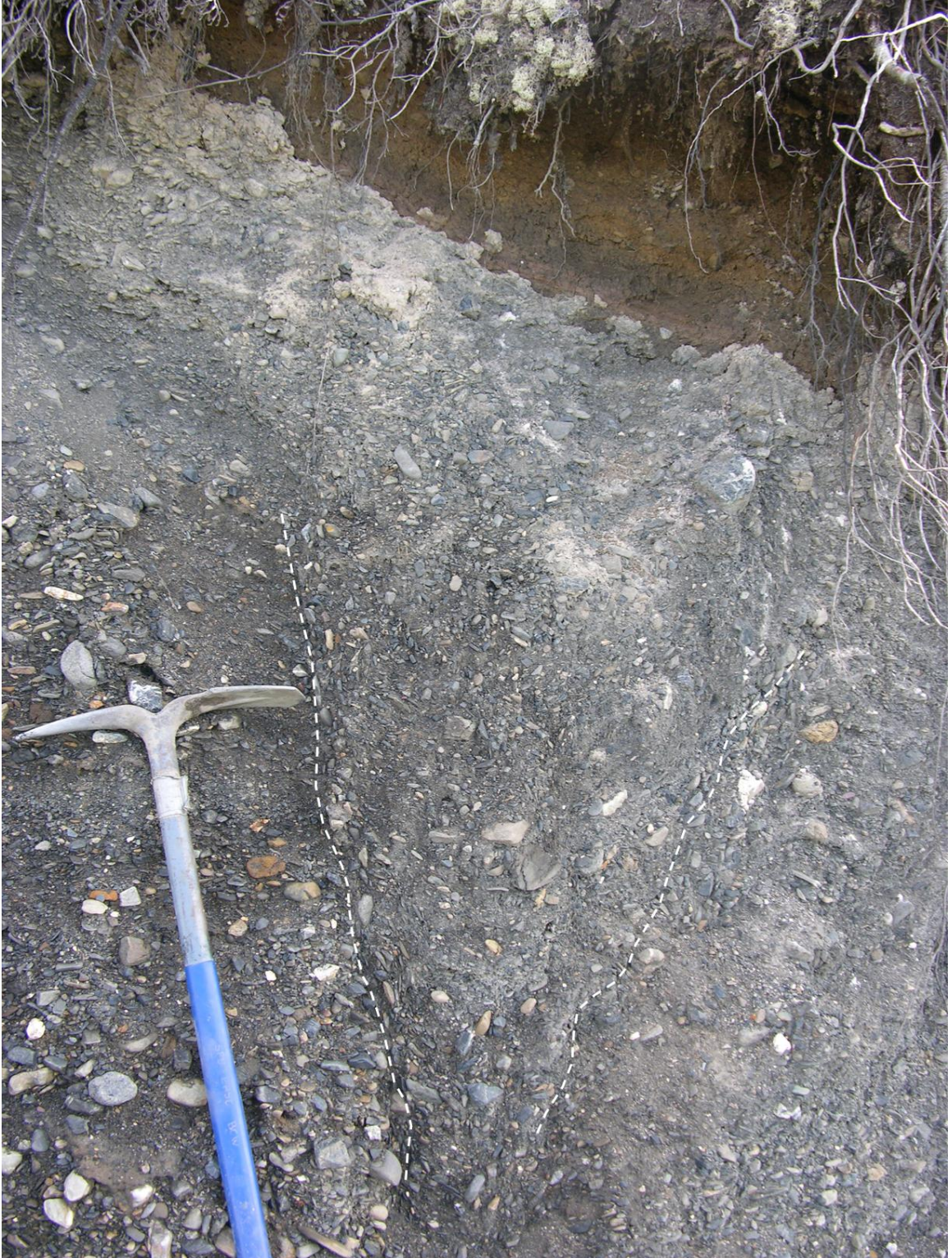
Figure 3.6 Ice wedge pseudomorph in glaciofluvial gravel at 07DT039.
