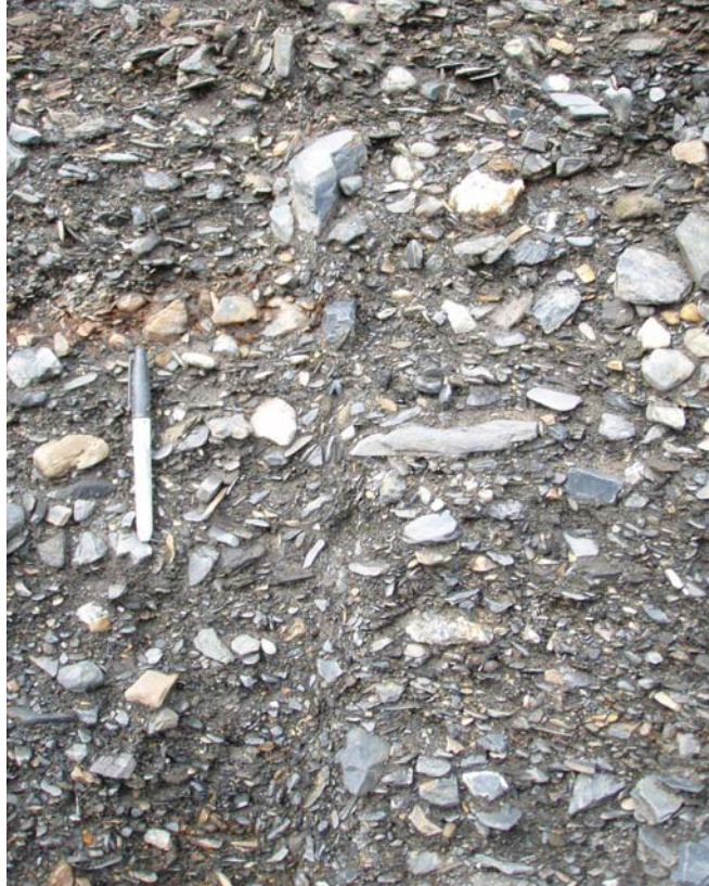
Figure 3.3 Glaciofluvial gravel, here exposed at 06DT133, typically form unit 1 across the study area. The sub-angular to well-rounded clasts are cemented in a sand matrix. Post-depositional normal faulting caused by loading has entrained the larger clasts. Pen is 14 cm.
