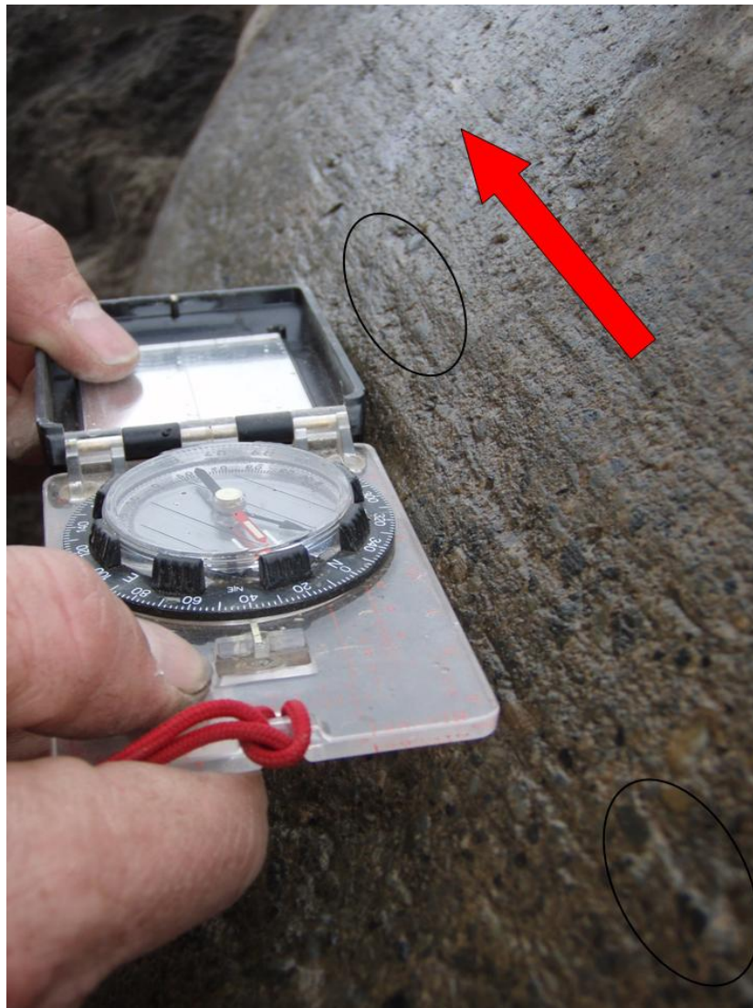
Figure 4.9 Rat tails on a 3-m-diameter boulder exhumed from the lower diamict unit at 07DT009 (Fig. 3.9). These rat tails correlate with till fabric measurements and indicate ice-flow to the southwest.
