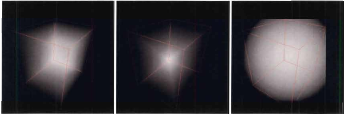
Figure 4.1: An illustration of the results for the three different methods of computing the per pixel rendering cost for a single brick. The brightness of each pixel represents the calculated rendering cost. From left to right: accurate method, backface method, and splatting method.
