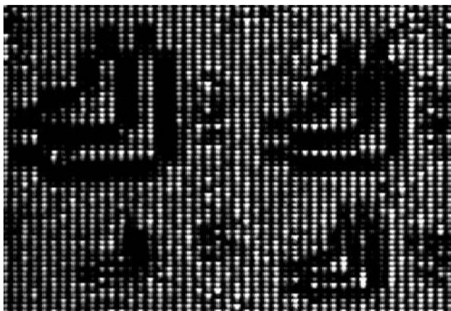
Figure 6-4 Small test structure (204 \mu\text{m} – 51 \mu\text{m} ) scans in 5 cm of water (Front position) at \lambda = 488\text{-}514 nm.
