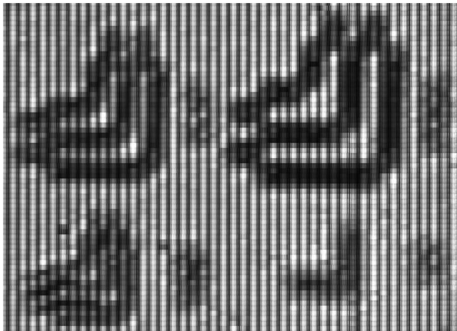
Figure 6-3 Small test structure (204 \mu\text{m} – 51 \mu\text{m} ) scans in 5 cm of water (Front position) at \lambda = 670 nm.
