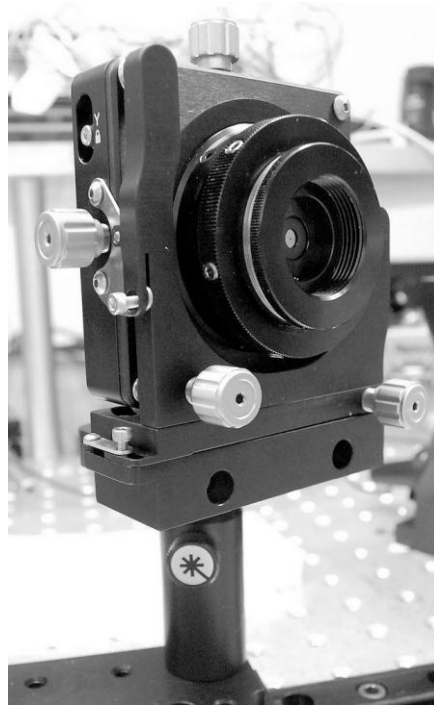
Figure 3-14 Photograph of the aperture mount (Multi-Axis Lens Positioner).
