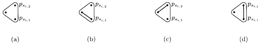
Figure 5.8: The clause gadget for clause C_i = p_{s_{i,1}} \vee p_{s_{i,2}} with two literals and all possible coverings. The coverings are depicted as solid edges joining particular pair of vertices. In (b), p_{s_{i,1}} has value 1 and p_{s_{i,2}} has value 0, in (c) p_{s_{i,1}} has value 0 and p_{s_{i,2}} has value 1, and in (d) both have value 1.
