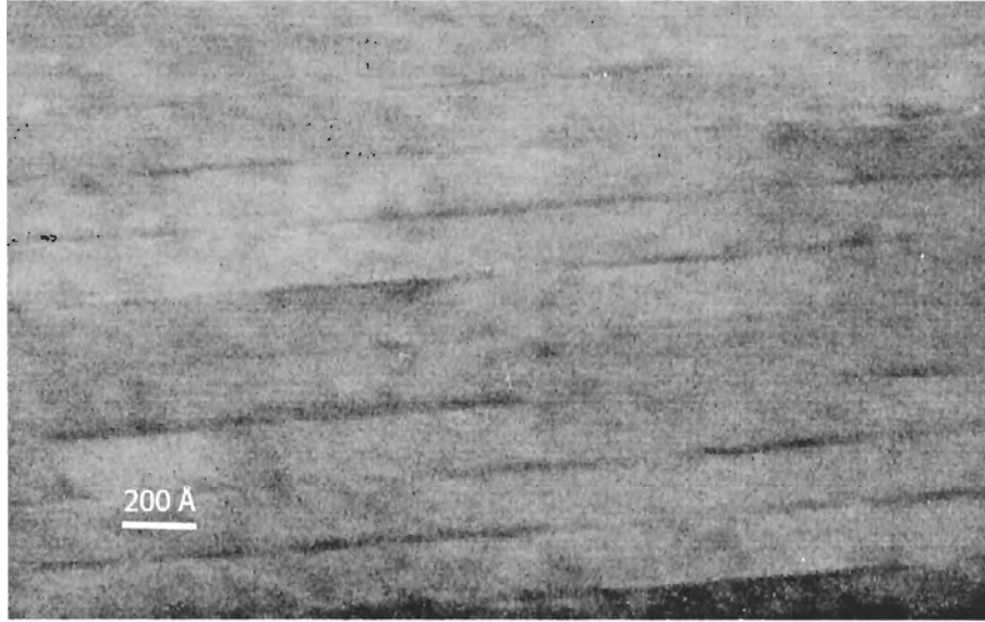
Figure 4.8: Cross-sectional TEM image of a MQW structure grown with the conventional growth sequence, showing 3D islands (thicker dark areas).
