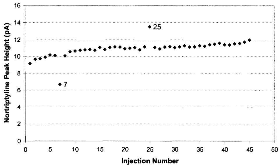
Figure 2.4: Plot of nortriptyline peak height (pA) versus injection number for a mid-range calibration standard containing 10 mg/L nortriptyline.
