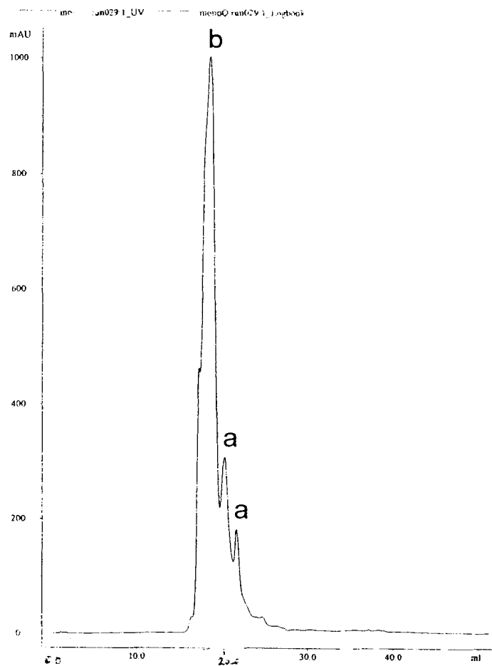
Figure 9. Separation of biotinylated peptide-MHC monomers by anion exchange. Fraction "b" extracted from the gel filtration procedure is run through an anion exchange column (MonoQ HR 5/5) by FPLC to separate the biotinylated from the unbiotinylated pMHC monomers. The eluent is collected in 1 ml fractions, which are subsequently tested in a biotinylation colour-change assay. Fractions labeled "a" are typically biotinylated, while those fractions that come off of the column earlier (b) are generally unbiotinylated.
