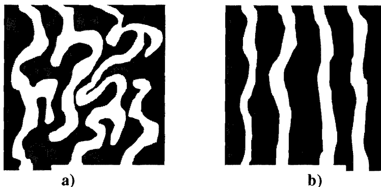
Figure 2.5 Connectivity of aqueous domains in PEMs (white = aqueous domains) where the degree of tortuosity of proton conduction pathway is greater in (a) than (b)
