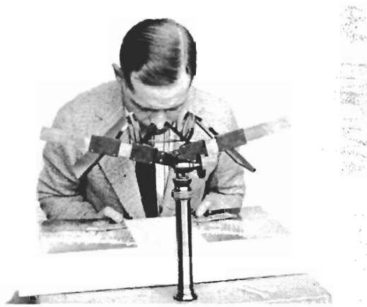
Figure 2.4: A viewer looking at a stereoscope that uses mirrors to project the two photographs to each eye separately so that the images are perceived in stereo. Photo courtesy of: US National Oceanic and Atmospheric Administration. Note: Copyright-free image. Retrieved from http://gimp-savvy.com/cgi-bin/img.cgi?noaaD3OKzLk1GHI4404 on March 1, 2007.
