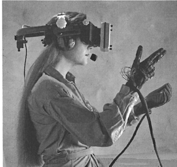
Figure 2.3: A user wearing a Head-Mounted Display (HMD) and using data gloves to interact with the display. Photo courtesy of NASA. Note: Copyright-free image. Retrieved from http://gimp-savvy.com/cgi-bin/img.cgi?ailsxmzVhD8OjEo694 on March 1, 2007.
