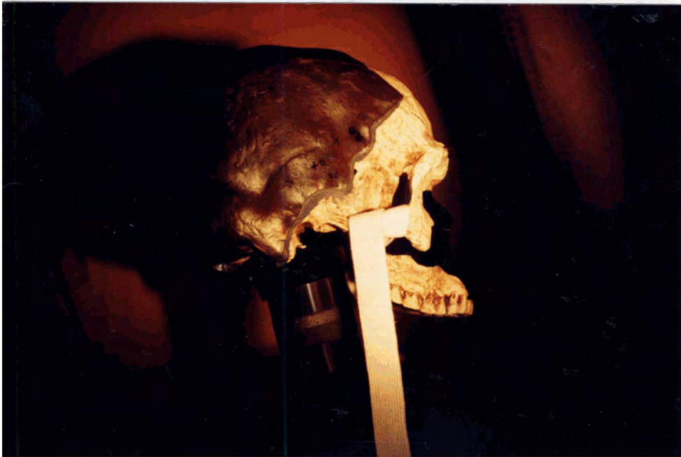
Figure 14: The Skhul V cranial cast under load, demonstrating the colour changes associated with a diffuse pattern of strain distribution.
