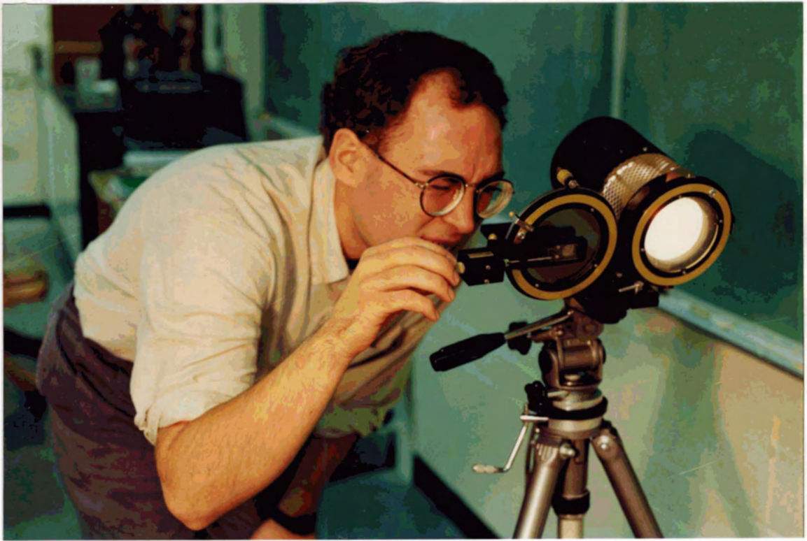
Figure 8 a and b: The polariscope, showing the use of the compensator. The right hand of the researcher is on this device, the aperture of which is positioned in front of the polarised filters.
