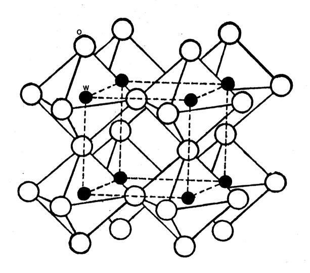
Fig. 2.3 The monoclinic WO $_3$  structure showing the distorted WO $_6$  octahedra projected along the y axis.
