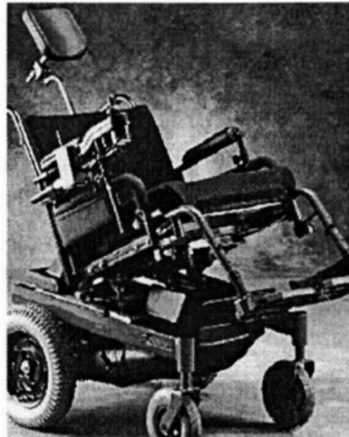
Figure 1.5: Invacare weight-shifting Tarsys tilt-in-space seat in tilted position. [26]
