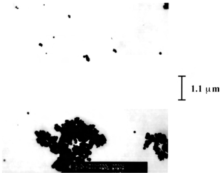
Figure 6.8 (b) TEM of PANI (10 wt%)-Nafion-Pt electrode.
