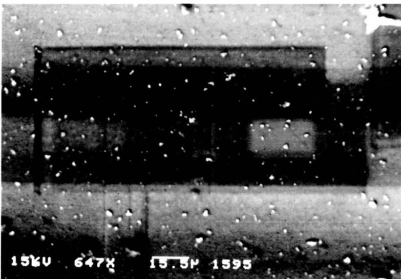
Figure 6.8 (a) SEM of PANI (10 wt %)-Nafion-Pt electrode.
