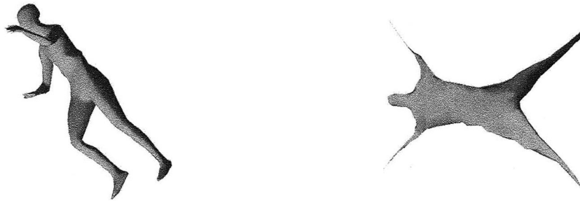
Figure 4.1: A human mesh (left) and its 3D spectral embedding, constructed using the second, third, and fourth eigenvectors. This particular choice of the eigenvectors is explained in Section 4.3.
