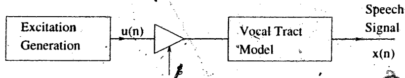
Figure 2.1: Simplified speech production model
