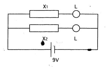
According to the brightness of two bulbs, reason and conclude about the different values of two resistors.
