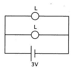
Give comments about the brightness of two bulbs in the circuit (b), and then compare the electrical characteristics of two bulbs.
