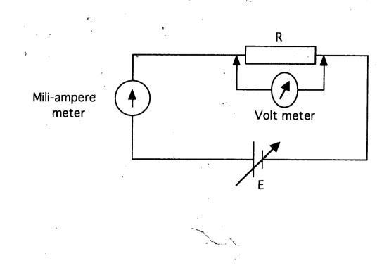
Vary the voltage difference of the power supply according to the following ranges: E1 = 3V, E2 = 5V, E3 = 6V, and E4 = 7.5V, and then take four different readings on the voltmeter and milli-ampere meter, and place them in the table below:
