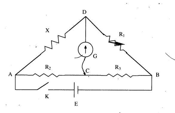
R1, R2 and R3 are the variable resistances, and X is unknown resistor.
