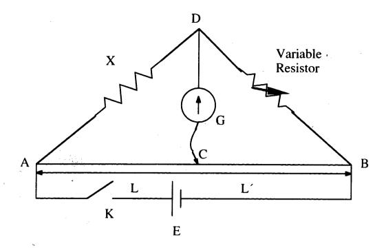
Move the alligator clip along the wire to find a point at which we have the zero-reading on the galvanometer. It is said that the Wheastone Bridge is balanced, and we have:
