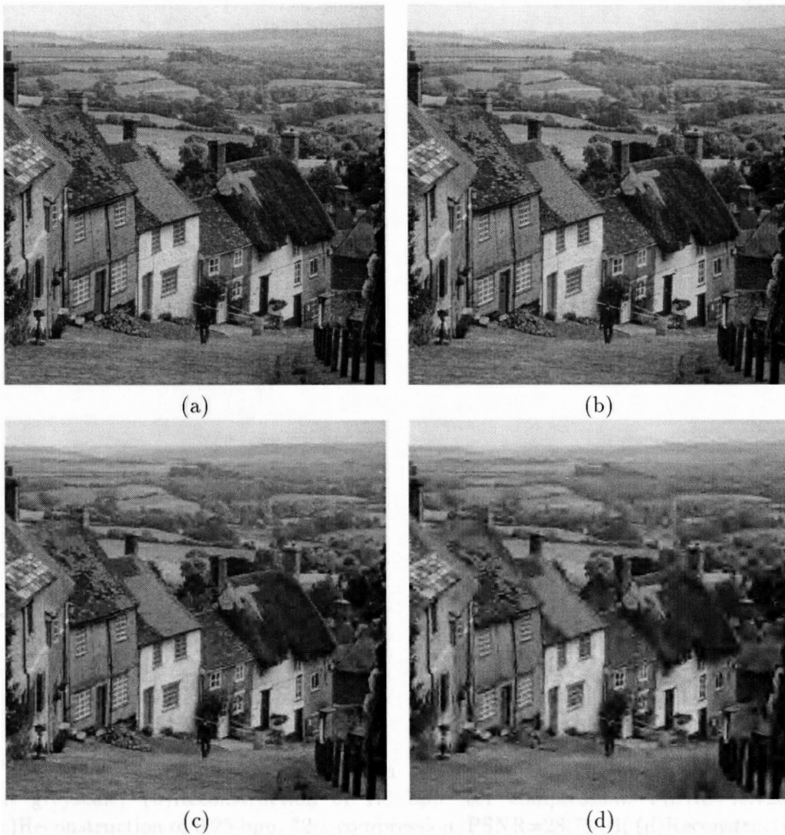
Figure 4.5: Result images of EZW on 'Goldhill', (a) Original image, 512 \times 512 8-bit greyscale; (b) Reconstruction of 1.0 bpp, 8:1 compression, PSNR=35.44dB; (c) Reconstruction of 0.25 bpp, 32:1 compression, PSNR=30.09dB; (d) Reconstruction of 0.10 bpp, 80:1 compression, PSNR=27.71dB
