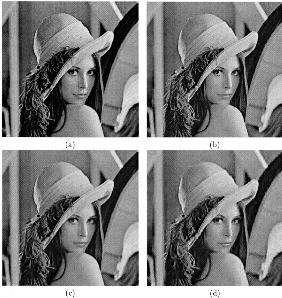
Figure 4.4: Result images of EZW on 'lena', (a) Original image, 512 \times 512 8-bit greyscale; (b) Reconstruction of 1.0 bpp, 8:1 compression, PSNR=39.31dB; (c) Reconstruction of 0.25 bpp, 32:1 compression, PSNR=33.15dB; (d) Reconstruction of 0.10 bpp, 80:1 compression, PSNR=29.50dB
