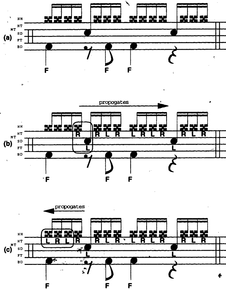
Figure 4.21: Another standard drum pattern is processed by the limb-assignment algorithm. In (a), hard-coded assignments, such as the foot pedals, are made in the first pass. In the second pass (b), notes within a certain distance in time (circled), are assigned to different limbs if the onsets are on different drums. The sixteenth notes at the beginning of the measure are skipped because they are the same drum, and a local onset has not been assigned to provide context. The sixteenth notes after the first snare hit are assigned since the first snare onset provides a starting point for alternating hands. In the third pass (c), notes within a certain distance in time (circled) are assigned, propagating changes backwards through the score.
