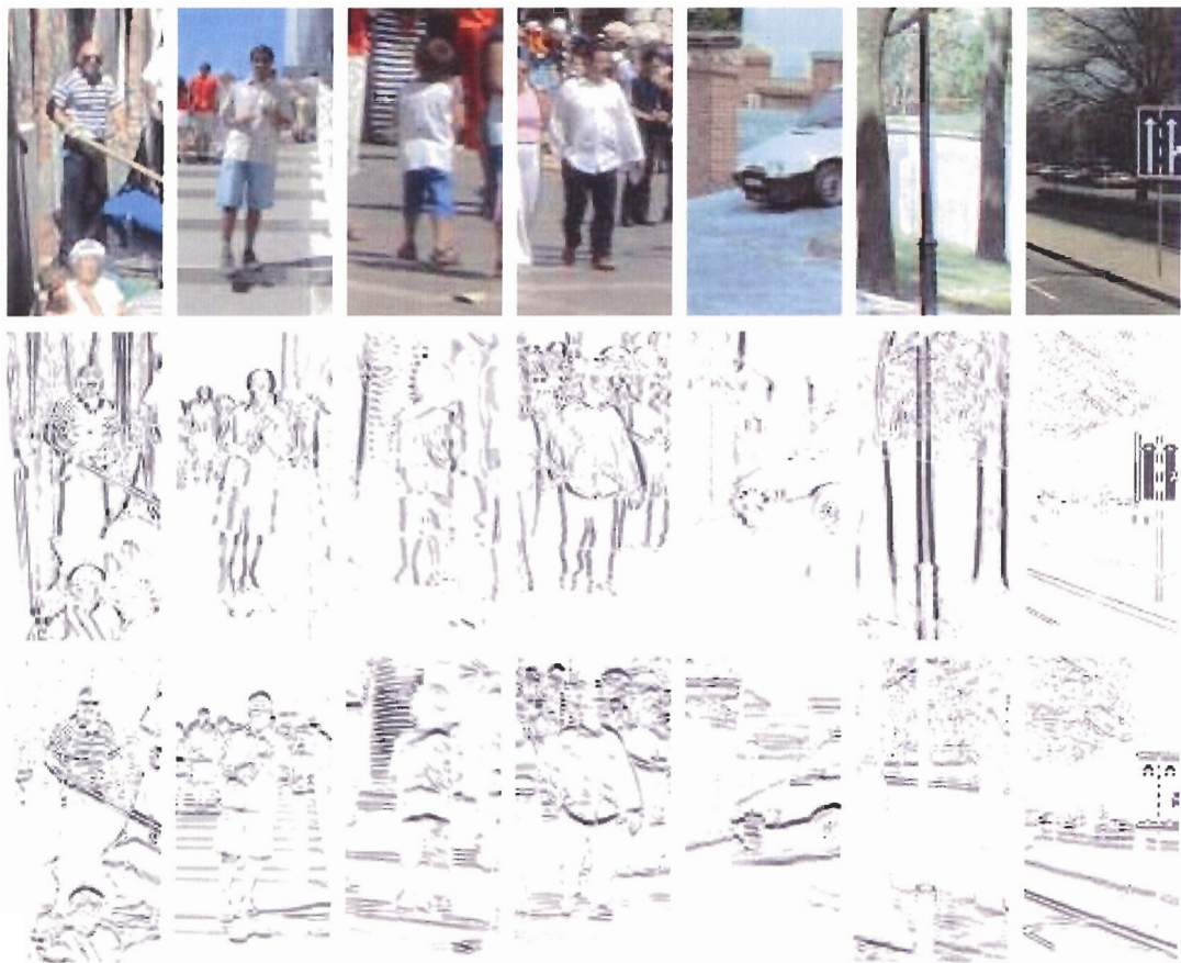
Figure 1.2: Examples of pedestrian and non-pedestrian images from our training set and their intensity gradients in x and y directions.
