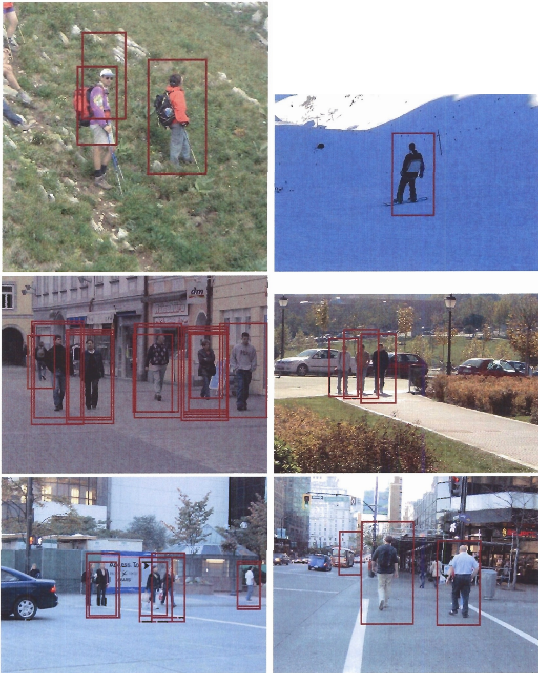
Figure 4.12: Results of running the detector on some of the test images. The multiple detections are because of multi-scale search, and one pedestrian might be detected in different scales. Some non-pedestrians are also falsely detected as pedestrians (false positives) in some of the images.
