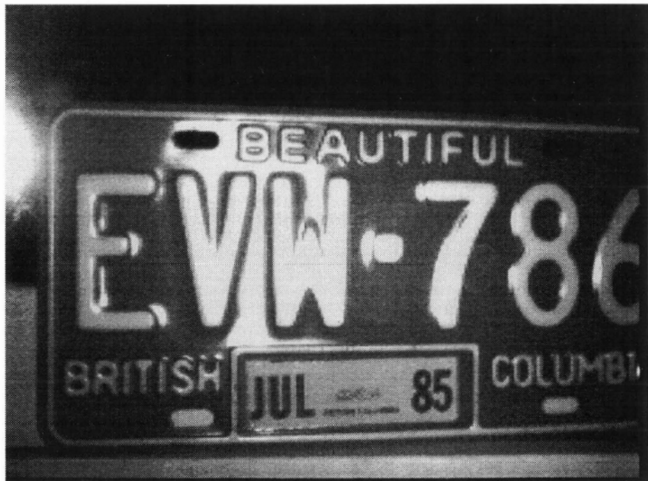
Figure 3.15 Image quality improvement a. before and b. after global adaptation: Yellow photochrome in B-725 matrix, PL #20; MOD – 420 nm
