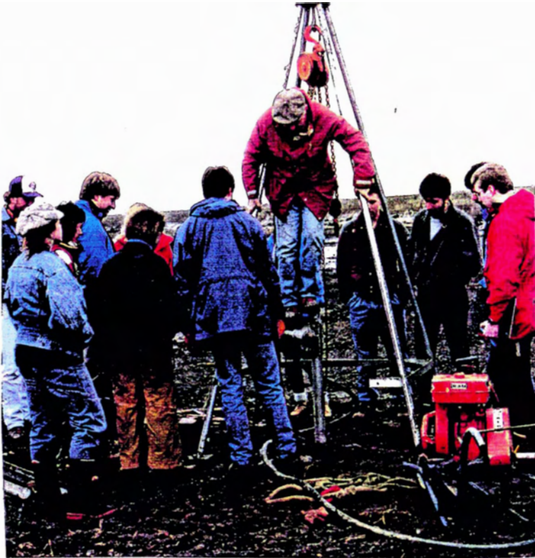
Figure 3.4 The large vibracorer in use, showing the derrick.
