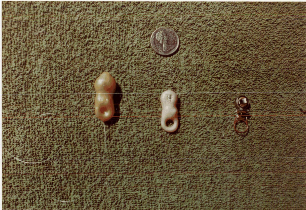
PLATE 3. Miniature radio transmitters used in migration studies.
