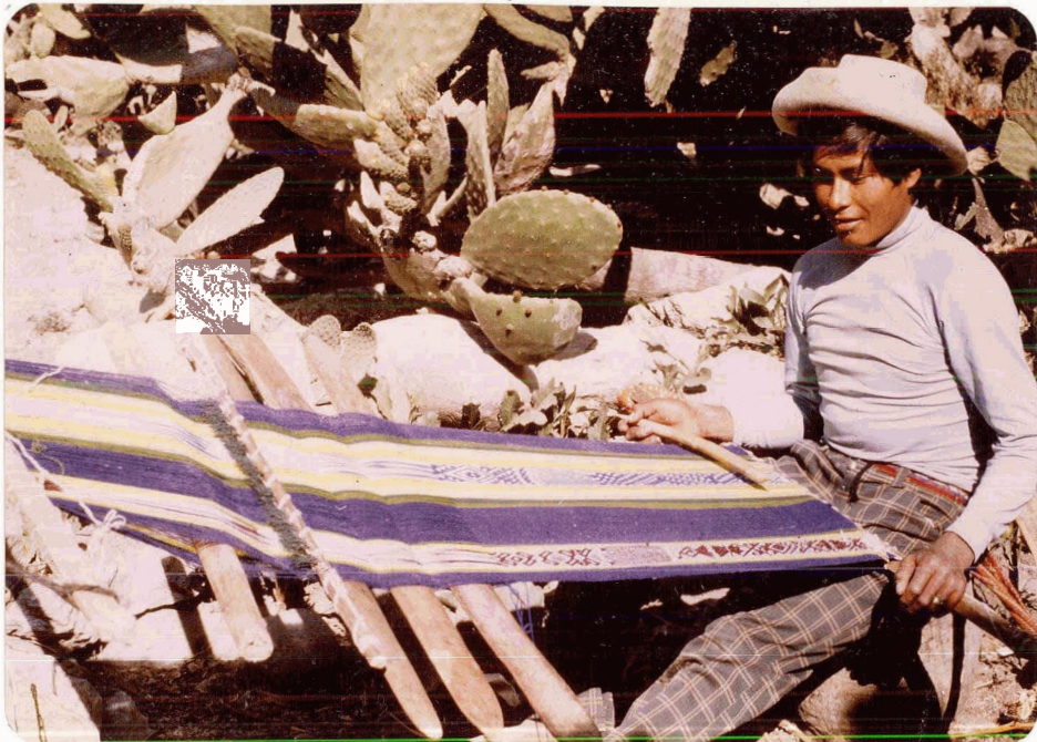
Figure 38. Stickloom with woven textile unwound from front end stick to show warp-faced designs
