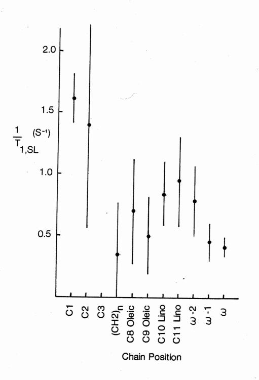
Figure 37. <sup>13</sup>C NMR spin label-induced spin-lattice relaxation rate due to 1.7 mol% 5-doxyl cholesteryl palmitate at 100.6 MHz and 46 °C. Uncertainties were calculated as in Figure 36.
