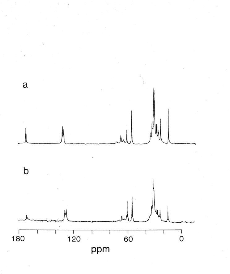
Figure 33. Proton decoupled <sup>13</sup>C NMR spectra of 20% W/V egg phosphatidylcholine vesicles in <sup>2</sup>H<sub>2</sub>O at 100.6 MHz and 46 °C (a) egg PC only (b) egg PC + ~ 1.7 mol% 5-doxyl cholesteryl palmitate. Inset indicates expansion of carbonyl region. Spectral parameters: Sweep width = 20 kHz; number of acquisitions = 1024; dataset = 32k; line broadening = 1.5 Hz; pulse width = 25 us (90° flip angle).
