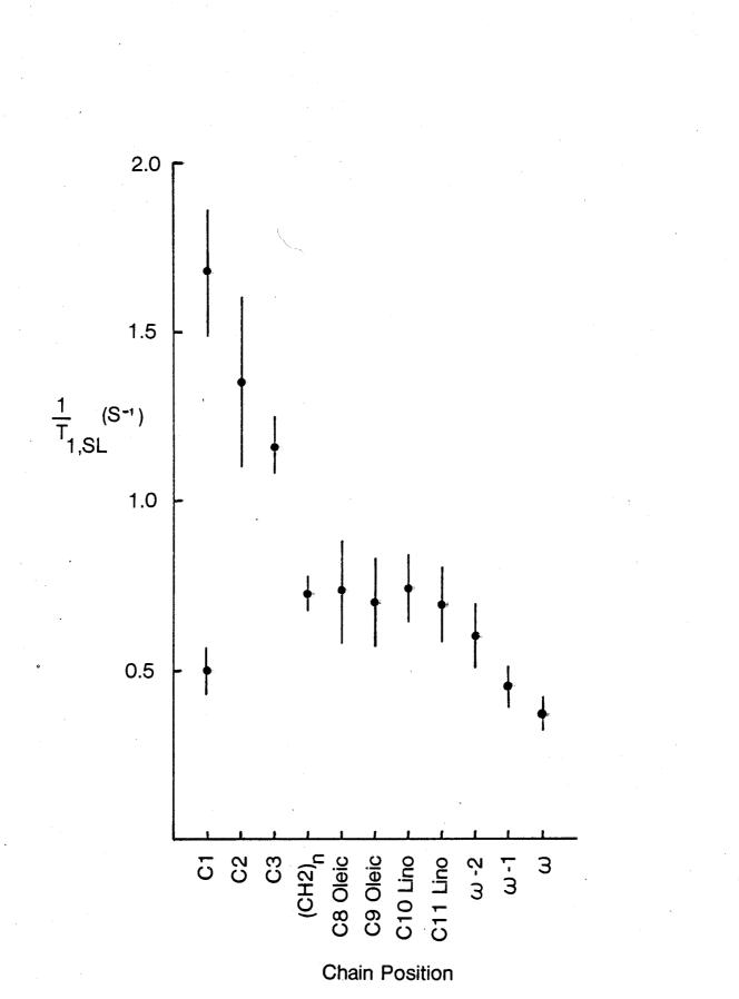
experimental error. Figures 32B and 33B indicate that, as expected, the linewidths of the acyl chain resonances are increased by the presence of the spin label in qualitatively the same pattern.
