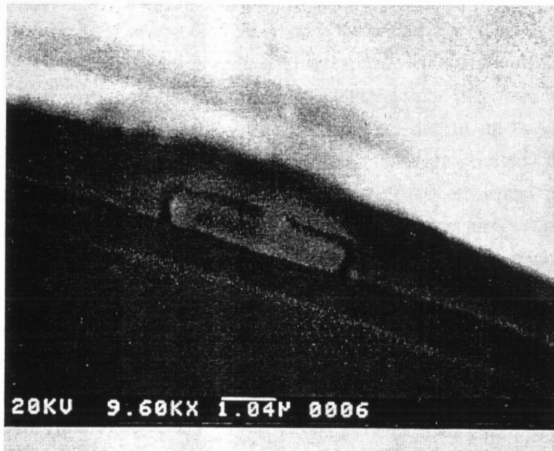
Figure 4.1 - SEM photograph of the cross-section of a beam-type polysilicon resistor.
