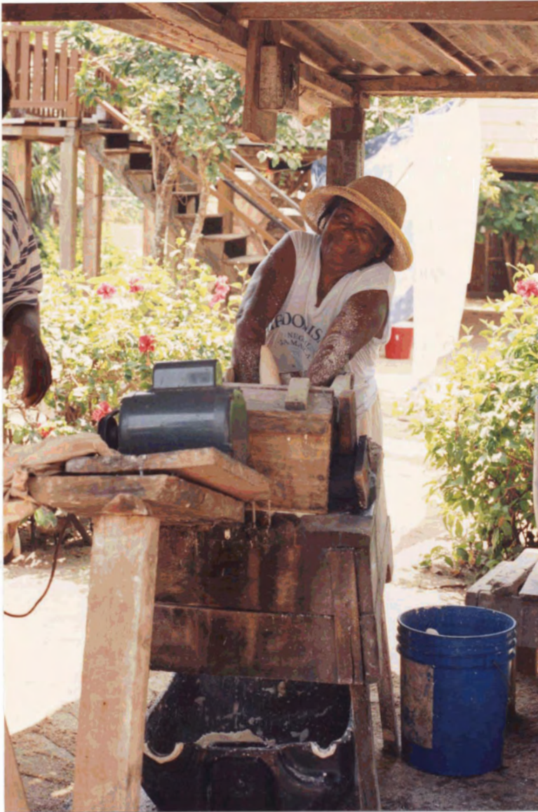
Figure 5.10: A Garinagu woman using a motor-driven cassava grater
