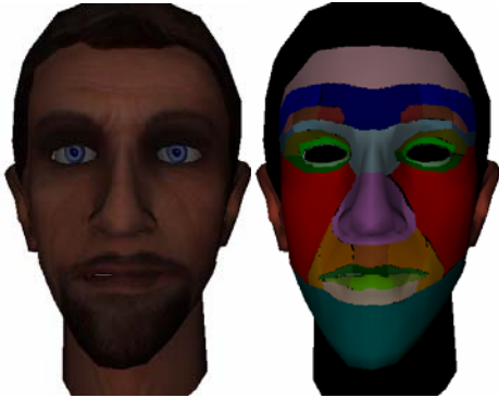
Figure 5. Face Regions. These are small areas that usually move together and are controlled by Feature Points. iFACE Components are related groups of these Regions, e.g. eye area
