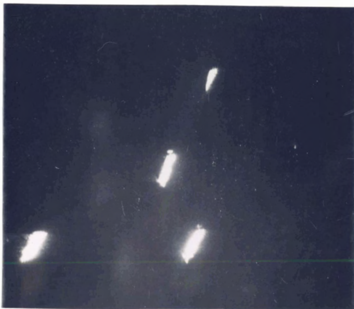
Figure 47: Polaroid photograph of the Bragg peaks. The peaks are at 11874eV, 12156eV, 12462eV and 12585eV.
