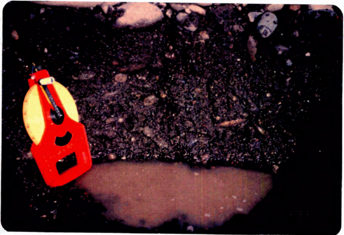
Fig. 4.2. Photograph showing (a) armoured gravel bar surface near the right bank and (b) composition of subsurface clastic sediments at the centre of the gravel bar on the Fraser River at Marguerite station.
