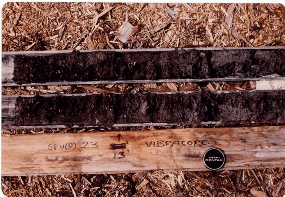
Figure 6.8 Organic-rich silt, core D23 (depth = 3.9 m below surface)
