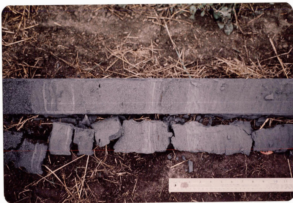
Figure 6.10 Interbedded silts and sands (top of core is to the right), core D25 (depth approx. 8 m)
