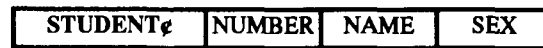
Figure A-2: Representation of the entity type STUDENT together with its properties NAME , NUMBER , and SEX .
