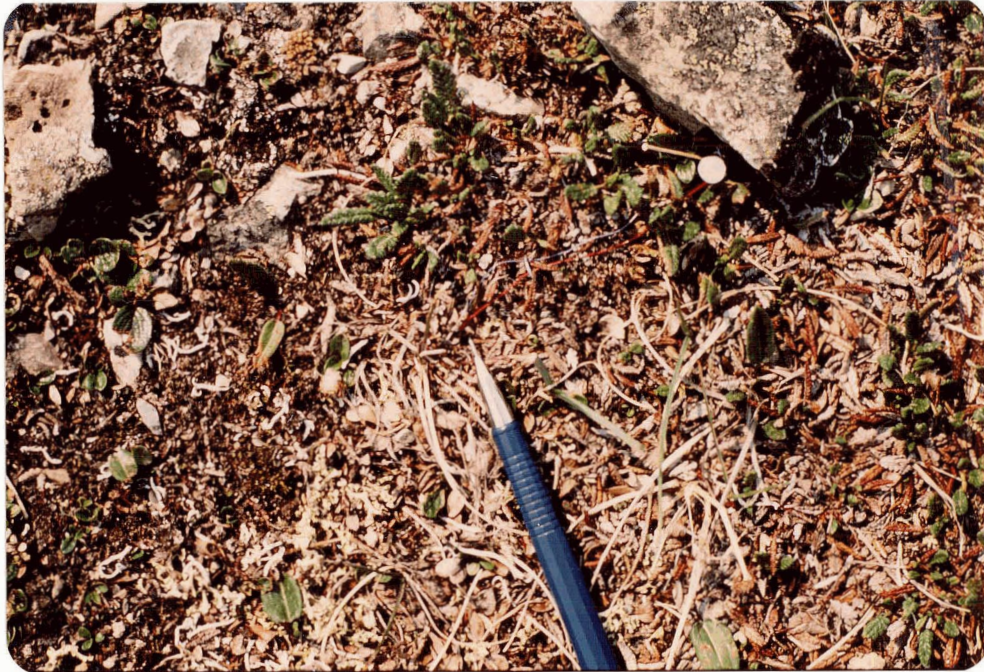
Figure 3.7. Photograph of single thermocouple junction of surface temperature array. Pencil pointing to thermocouple junction indicates scale.
