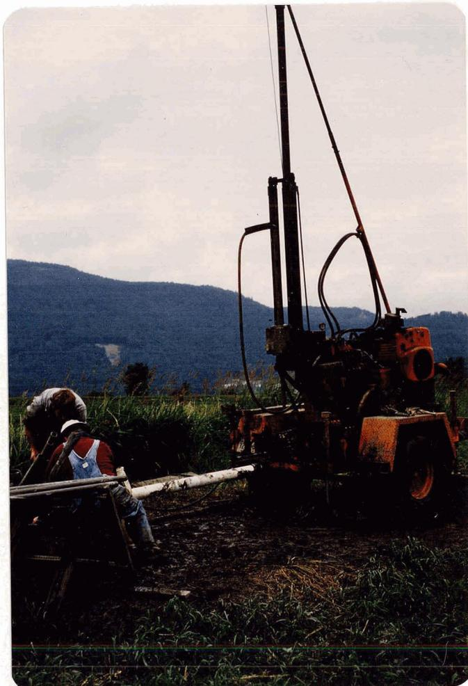
Fig. 2.0 Concore C-68 Drill Rig
