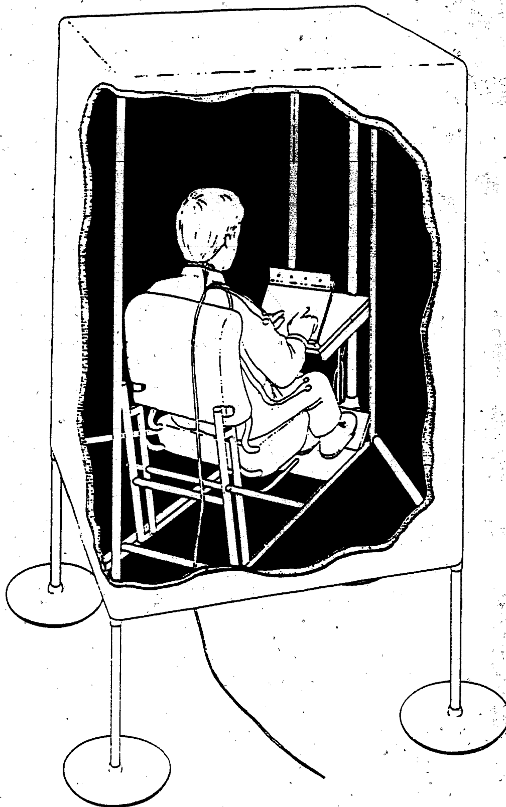
Figure 2.3: Experimental set-up for the hot air exposure study. Subjects remained seated in a helicopter pilot seat suspended within an environmental chamber. Evaporative rate through the clothing was monitored by means of Vapour Flow Meters positioned on the arm, chest and thigh.
